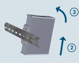
Press the top of the Data Diode towards the DIN rail until it snaps into position.
