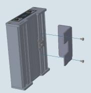
The DD1G Gen 2 Data Diode comes with a DIN rail bracket intended for vertical DIN rail mounting. It must be mounted on the device before use.
