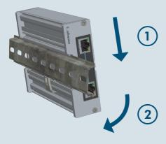
Fit the groove above the DIN rail clip on the Data Diode to the upper edge of the DIN rail.
