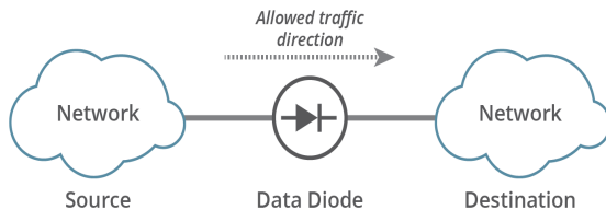
Figure 5 - Data Diode traffic direction.
