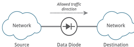
Figure 7 - Data Diode traffic direction.
